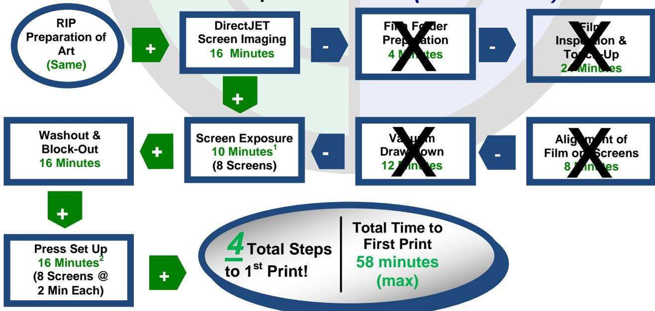
1. The lack of film, glass and vacuum drawdown eliminates pinhole re-touching and overall screen making time.
