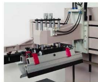
自由水平浮動之印刷座 Pneumatic Lift-up of Print Head
